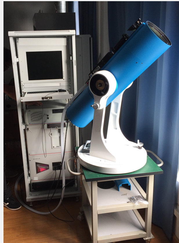
Figure 1. DIAL systems use two lasers with different frequencies to observe absorption differentials, allowing the detection and measurement of airborne pollutants
